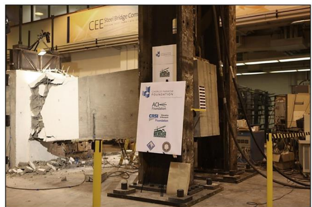
Figure 49. Section of the RC beam tested and global view of the test specimen and setup at 5.5% drift with plastic hinge failure in shear and bar buckling.
